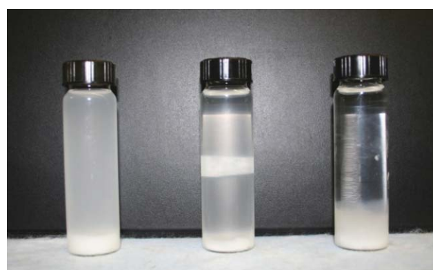
Fig. 8 Suspensions of cellulose nanocrystals showing gradual aggregation of cellulose nanocrystals with time.
