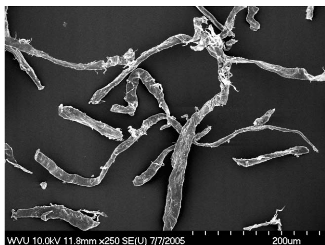
Fig. 1 Scanning electron micrograph showing recycled pulp before cellulose hydrolysis.
